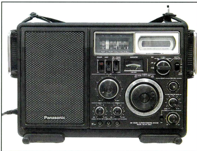
Photo B. The Panasonic RF-2800 was an early PLL portable that featured digital frequency readout at an affordable price. (Courtesy of RigReference.com < http://bit.ly/VqVrcO >)
